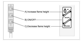
Figure 23: Switch Panel and Wall Switch/Touch Pad
