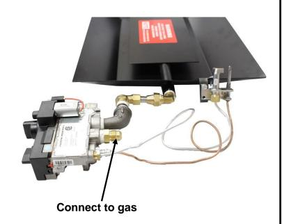
**IMPORTANT:** The minimum inlet supply pressure for the purpose of input adjustment is 5.0 inches (natural gas) 11 inches (propane gas) in water column. The maximum inlet supply pressure is 10.5 inches (natural gas) 13 inches (propane gas) in water column.
