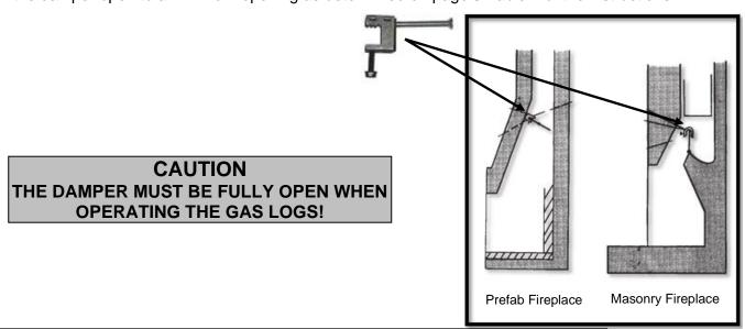
IMPORTANT: In the Commonwealth of Massachusetts the damper must be either permanently welded in the fully open position or completely removed.
