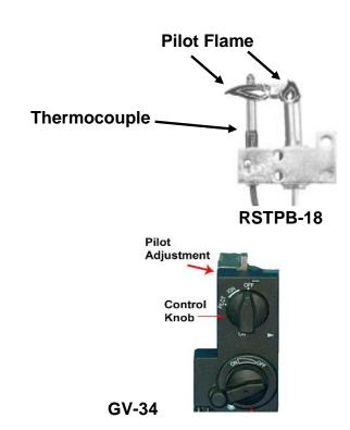
IMPORTANT: These controls are factory preset and will not normally require additional adjustment of the pilot flame. If field adjustment of the pilot flame is required, adjust using the pilot adjustment screw. The 90 degree pilot should produce 2 flames about 1-1 ½" in 2 directions. One flame should come towards the front of the firebox to ignite the burner and the other, wrapping around the thermocouple to ensure proper valve operation.
