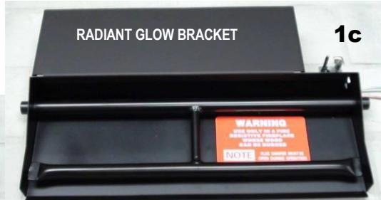
STEP 1: Figure 1a illustrates how the radiant glow bracket slides and rests on the back of the burner pan. For installation on burner pans without pilots center the bracket on the back of the burner pan as shown in figure 1b. For installation on burner pans with a pilot install the bracket on the back of the burner pan allowing 1" clearance around the pilot assembly as shown in figure 1c. The grate can then be pulled forward over the burner pan, as shown in figure 1e.
