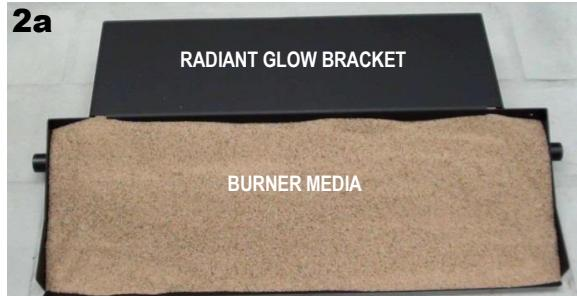
STEP 2: Fill the burner pan with the appropriate media as shown in figure 2a (sand for NG and vermiculite for LP) Install the grate over the burner pan. The front legs of the grate go around the burner pan and about 1" in front of the burner pipe as shown in figure 2b.
