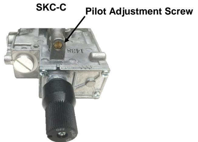
**IMPORTANT:** These controls are factory preset and will not normally require additional adjustment of the pilot flame. If field adjustment of the pilot flame is required, adjust using the pilot adjustment screw. The 90 degree pilot should produce 2 flames about 1-1 1/2" in 2 directions. One flame should come towards the front of the firebox to ignite the burner and the other, wrapping around the thermocouple to ensure proper valve operation.
