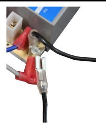
A RC-S12V-MV should be with this valve. Remove it and assemble it according to its instructions. Once assembled, connect the wires to the Grey wire from the Blue wire harness and the other wire to the module as shown.
