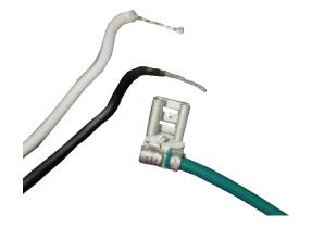
Connect the black and white wires from the transformer to a 110V plug and the Green wire to a ground.
