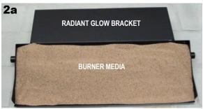
STEP 2: Fill the burner pan with the appropriate media as shown in figure 2a (sand for NG and vermiculite for LP) Install the grate over the burner pan. The front legs of the grate go around the burner pan and about 1" in front of the burner pipe as shown in figure 2b.
