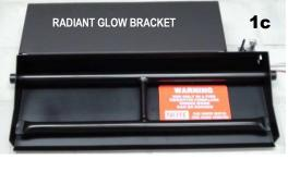
STEP 1: Figure 1a illustrates how the radiant glow bracket slides and rests on the back of the burner pan. For installation on burner pans without pilots center the bracket on the back of the burner pan as shown in figure 1b. For installation on burner pans with a pilot install the bracket on the back of the burner pan allowing 1" clearance around the pilot assembly as shown in figure 1c. The grate can then be pulled forward over the burner pan, as shown in figure 1e.
