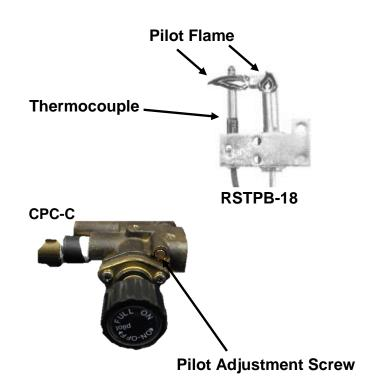
**IMPORTANT:** These controls are factory preset and will not normally require additional adjustment of the pilot flame. If field adjustment of the pilot flame is required, adjust using the pilot adjustment screw. The 90 degree pilot should produce 2 flames about 1-1 1/2" in 2 directions. One flame should come towards the front of the firebox to ignite the burner and the other, wrapping around the thermocouple to ensure proper valve operation.
