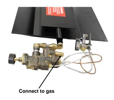
**IMPORTANT:** The minimum inlet supply pressure for the purpose of input adjustment is 5.0 inches (natural gas) 11 inches (propane gas) in water column. The maximum inlet supply pressure is 10.5 inches (natural gas) 13 inches (propane gas) in water column.
