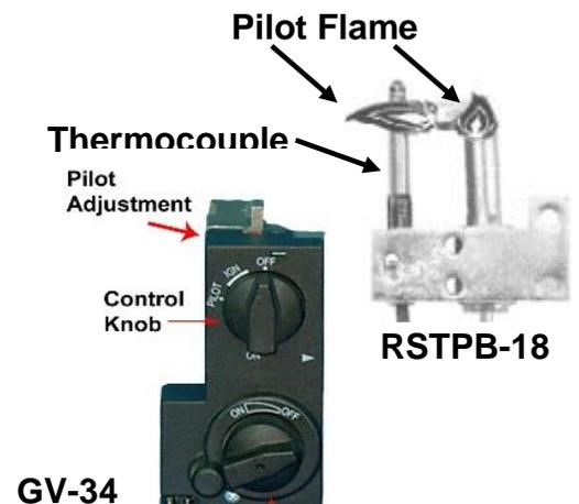
**IMPORTANT:** These controls are factory preset and will not normally require additional adjustment of the pilot flame. If field adjustment of the pilot flame is required, adjust using the pilot adjustment screw. The 90 degree pilot should produce 2 flames about 1-1 ½" in 2 directions. One flame should come towards the front of the firebox to ignite the burner and the other, wrapping around the thermocouple to ensure proper valve operation.
