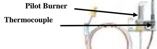
5. Turn knob on gas control counter-clockwise to "PILOT".
