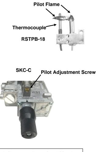
**IMPORTANT:** These controls are factory preset and will not normally require additional adjustment of the pilot flame. If field adjustment of the pilot flame is required, adjust using the pilot adjustment screw. The 90 degree pilot should produce 2 flames about 1-1 ½" in 2 directions. One flame should come towards the front of the firebox to ignite the burner and the other, wrapping around the thermocouple to ensure proper valve operation.
