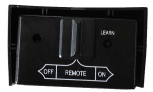
**IMPORTANT**: Keep receiver in a cool location. Battery life is also significantly shortened if batteries are exposed to high temperatures. Make sure the remote receiver switch is in the OFF position. For best results it is recommended that 18 gauge stranded wires should be used to make connections and no longer than 20-feet.
