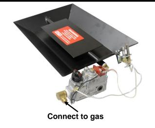
**IMPORTANT:** The minimum inlet supply pressure for the purpose of input adjustment is 5.0 inches (natural gas) 11 inches (propane gas) in water column. The maximum inlet supply pressure is 10.5 inches (natural gas) 13 inches (propane gas) in water column.
