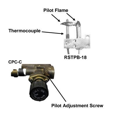
**IMPORTANT:** These controls are factory preset and will not normally require additional adjustment of the pilot flame. If field adjustment of the pilot flame is required, adjust using the pilot adjustment screw. The 90 degree pilot should produce 2 flames about 1-1  $\frac{1}{2}$ " in 2 directions. One flame should come towards the front of the firebox to ignite the burner and the other, wrapping around the thermocouple to ensure proper valve operation.
